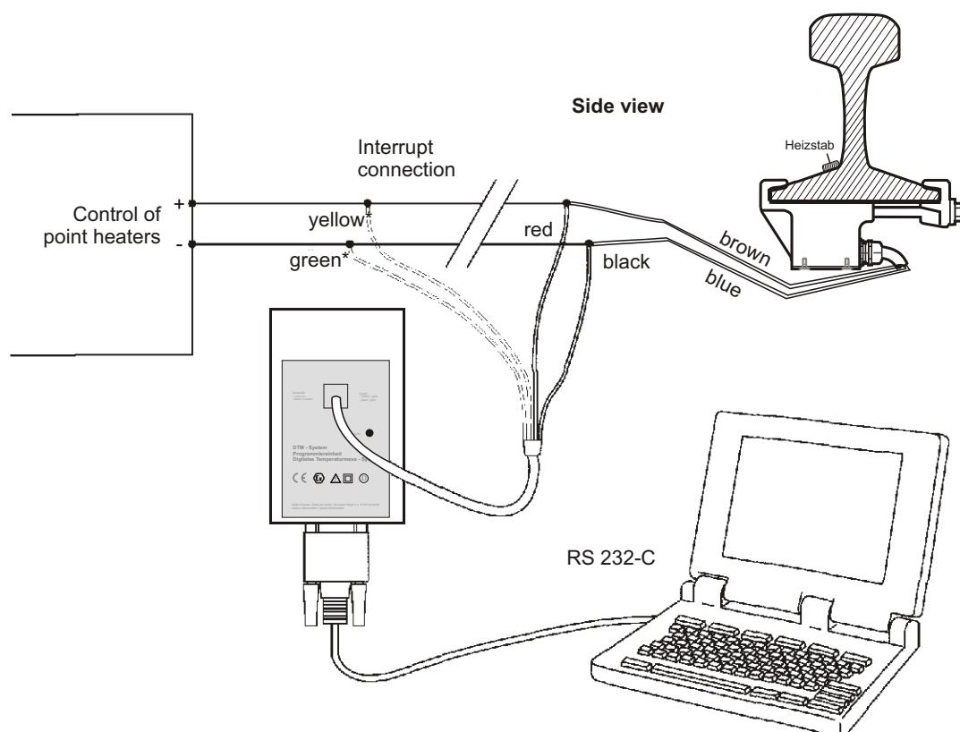
Attention : "yellow \*" and "green \*" are only to be connected if the digital temperature measurement recorder is to be configured during running operation.
